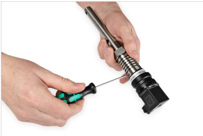
Disconnect the electronic unit by loosening the threaded union or the two set screws.
