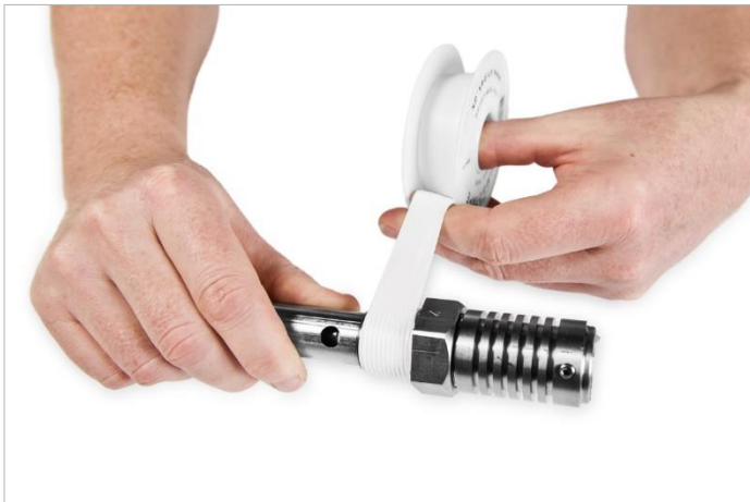
Apply Teflon tape or liquid gasket on sensors with a conical thread. For other thread types, a washer is used.
