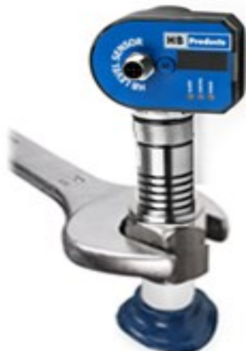
Mount the sensor on the vessel. Torque 80-150 Nm.
