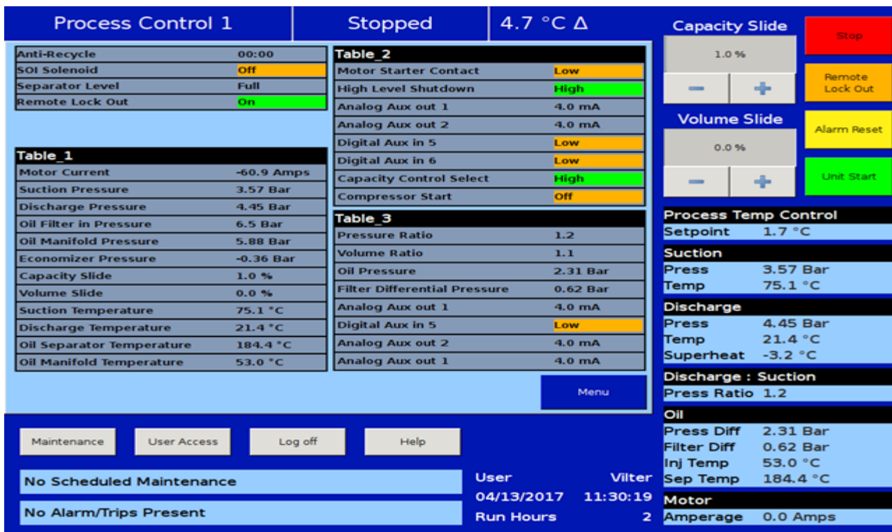
Figure 4-11. Configurable Main Screen with SOI Solenoid and Separator Level
