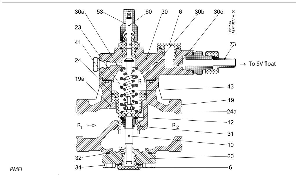
When the liquid level inside the float drops, the float orifice opens. This relieves the higher pressure,  $p_s$ , acting on the servo piston to the low pressure side causing the PMFL to open. Variations in liquid level will result in variations
