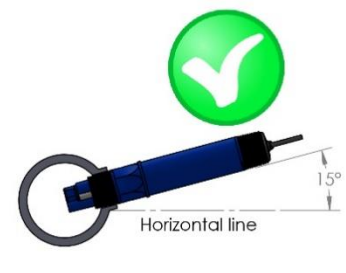
Horizontal pipe installation
