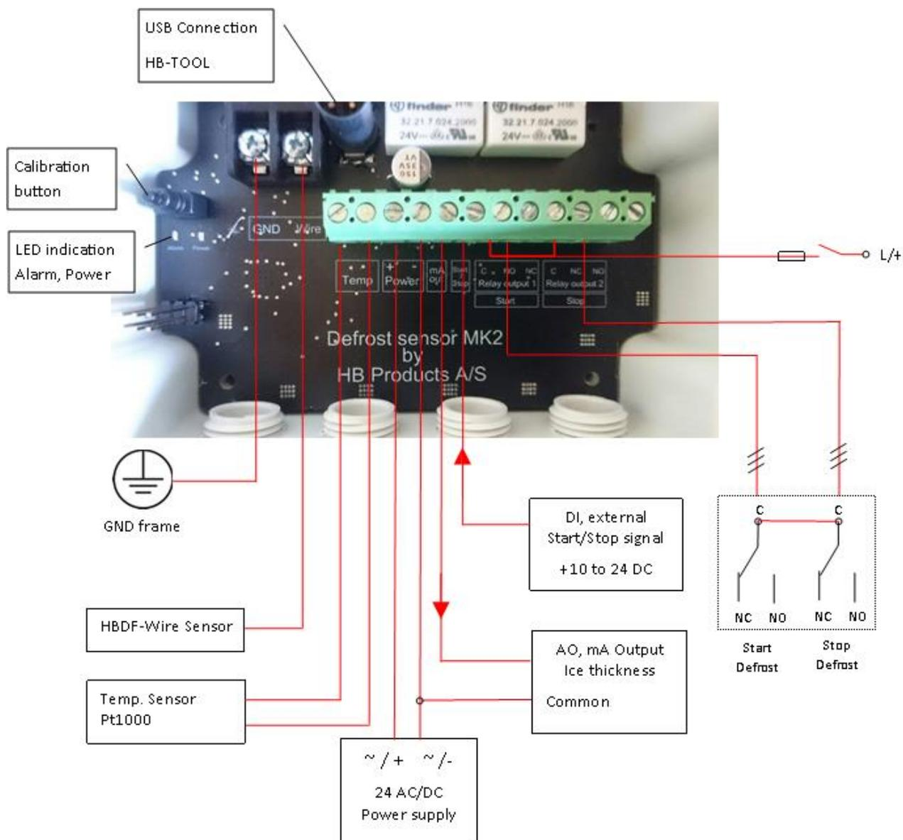
**Simple defrost with electric heater.**
