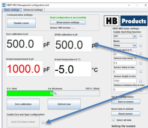
When the sensor is installed and the evaporator is dry and without ice, connect the sensor to the HB-tool using a USB cable.
