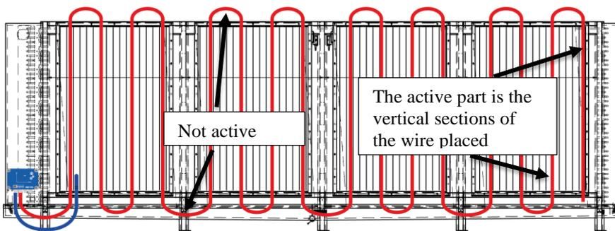
The temperature sensor should be placed where ice melt slowly. Keep away from the hot tubes or electrical elements used for defrosting.
