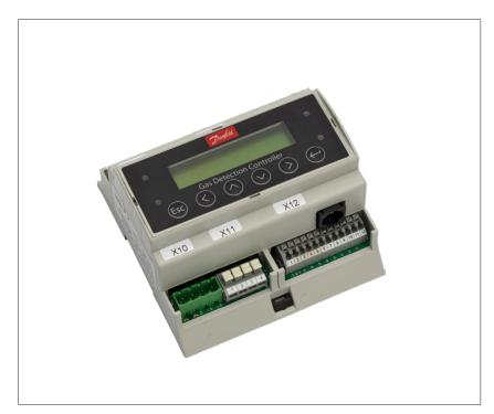
The gas detection Controller Unit is used for a centralized monitoring and warning of hazardous gas concentrations. The input signals for the controller are collected from the local gas detection units of the types Basic, Premium and Heavy Duty via RS485 Fieldbus or Analog communication. In total 96 gas detection sensors can be handled via Fieldbus + 4 via Analog directly on the controller (+28 additional possible if expansion modules added).
