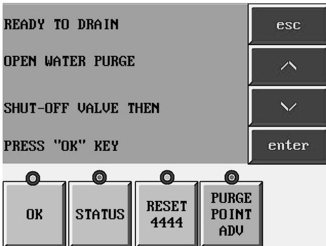
**Ready to Drain Water** – appears when the concentrating water process has been completed and water is ready to be drained.
