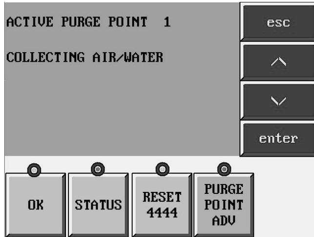
**Collecting Air/Water** – appears when the APPT is in its normal operating of collecting noncondensable gas and water.
