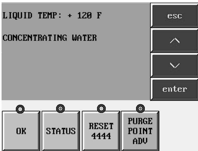
**Concentrating Water Mode** – appears during the process of heating the ammonia/water solution to remove as much ammonia from the water as possible before releasing the water. The liquid temperature appears during the concentrating water mode to indicate the temperature of the ammonia/water solution (units will match the selected display units).
