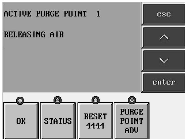
**Releasing Air** – appears when the APPT is releasing noncondensable gas.
