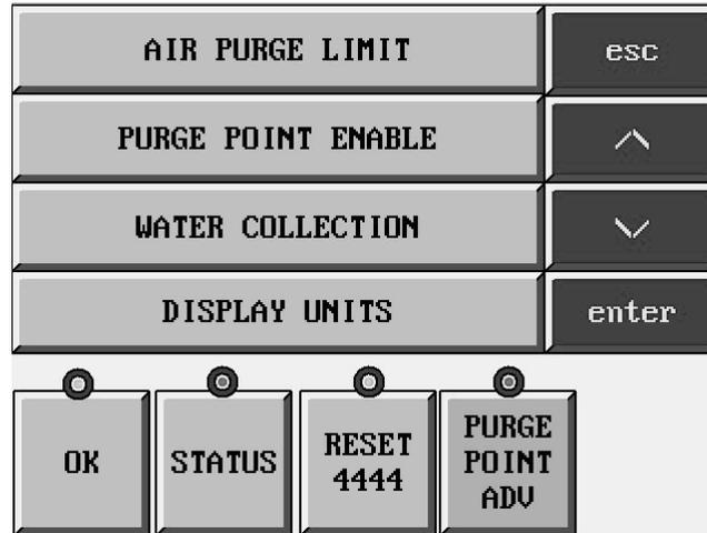
Along the bottom of the control console there are four functional keys for specific tasks. Each will have a green dot above it when the key is available and a red dot above it when the key is unavailable.
