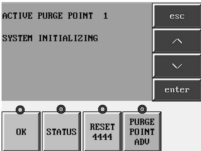
**System Initializing** – appears after either the System Reset key has been pressed or power is cycled to the APPT while the Liquid Make-Up Level Sensor is reading wet. APPT will stay in this mode until Liquid make-Up Level Sensor reads dry. This prevents the heaters from turning on until the evaporator shell has filled with liquid.
