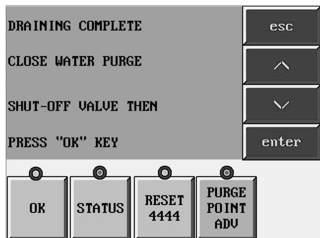
**Draining Complete** – appears when the APPT is done draining and is ready to go back to its normal mode, Collecting Air/Water
