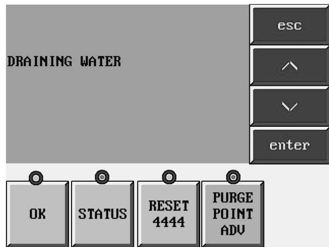
**Draining Water** – appears when the concentrated water is draining from the APPT.
